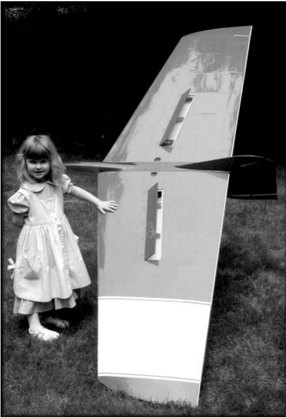
Underside of the Blackbird XC with flaps fully deflected. Granddaughter Anna, age three and a half, provides some scale.
