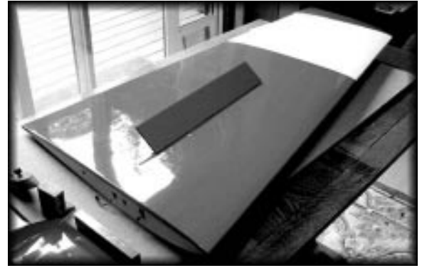
Bottom of the right wing after the covering was applied. The flap recess has not been cut out yet, so the hinges are not connected. Each flap is over fifty square inches in area, so substantial servo power is required.
