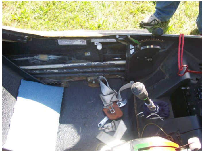
Left arm rest removed exposing flap and spoiler drive rods and belt attachment.
