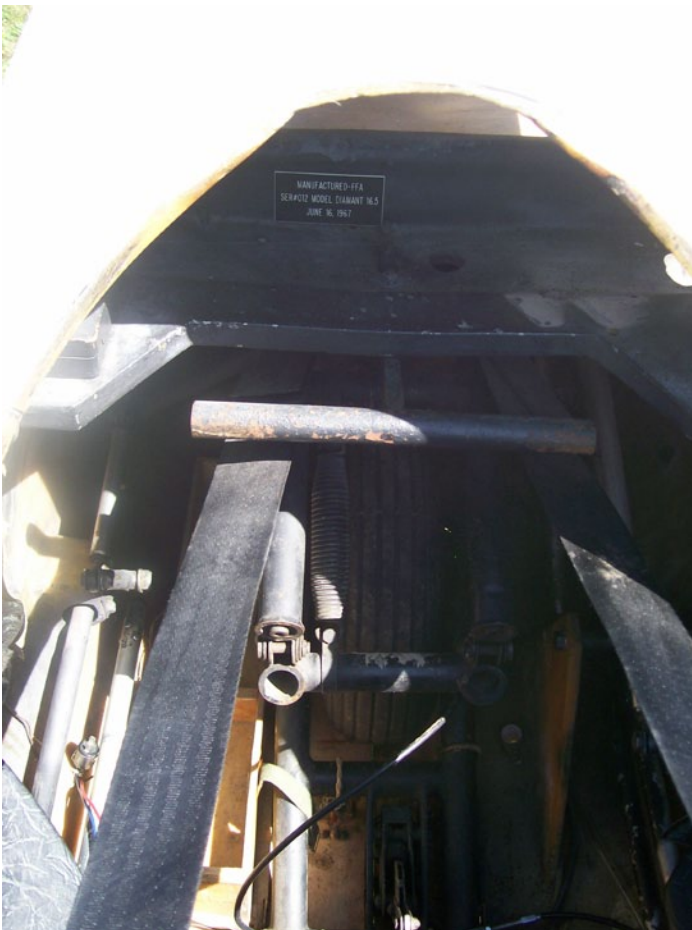
Left: Seat back removed, aircraft data plate Above: Spoiler, aileron and flap connection points on the inside
