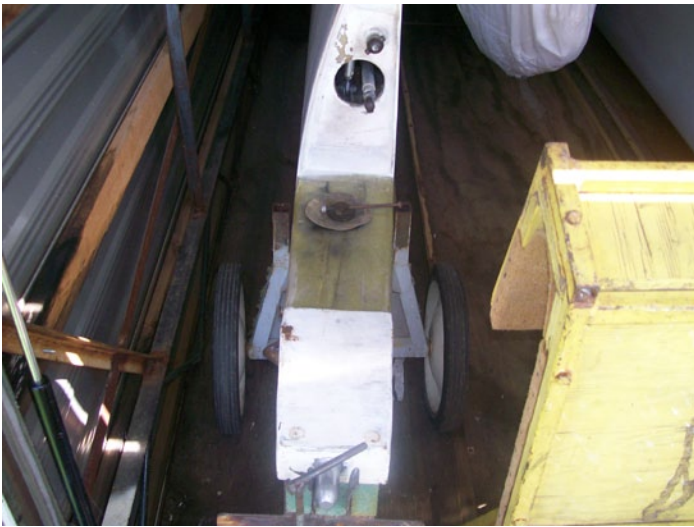
Right wing root secure point note the tie pin through the main wing pin hole.
