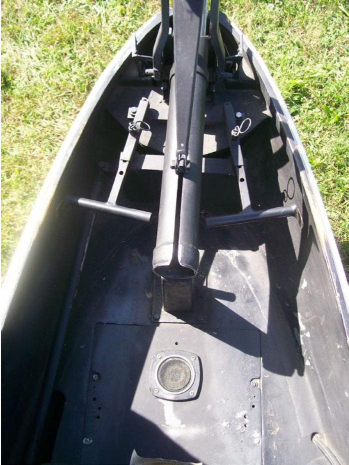
Rudder pushrod on left, vario speaker in center canopy slide on the top and rudder pedals in the front.
