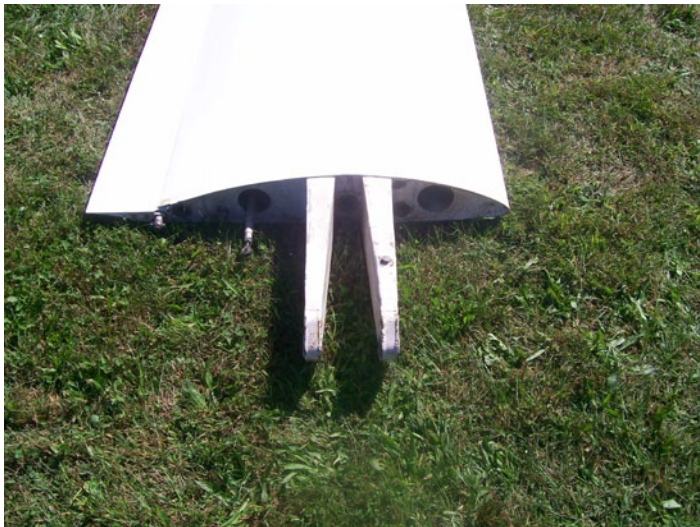
Left wing root showing off Y-spar and control connections.
