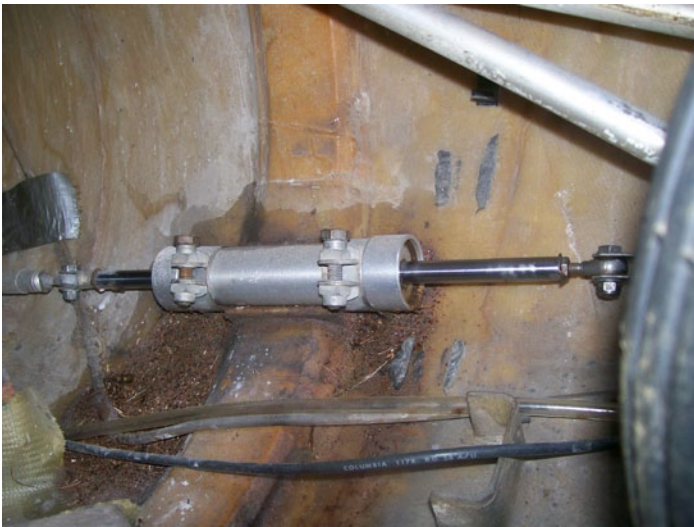
Rudder damper prevents high speed flutter of the rudder.
