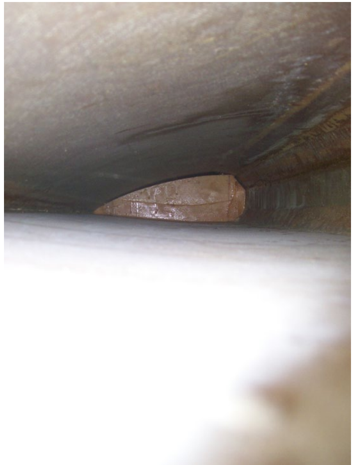
Right Wing leading edge D-tube fewer glue runs on this side.
