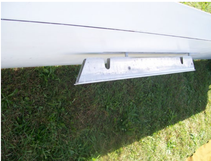
Below right: Trailing edge view of lower left wing showing spoiler extended and flaps in negative position.
