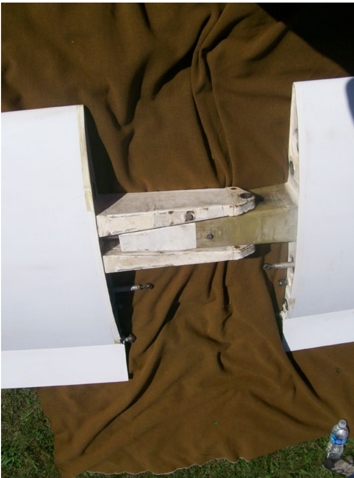
Above: Inside the leading edge of the left wing. Look Ma, no ribs! Wing spar is to the left.
