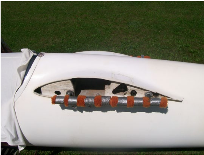
Left wing pin covers in place.
