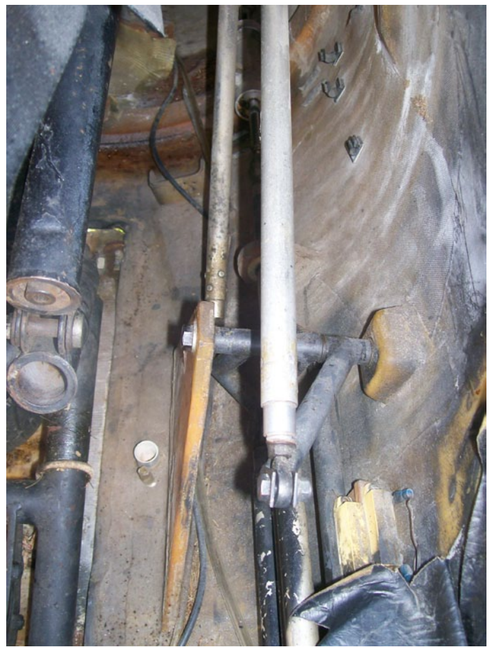
Flap and spoiler drive rods and mountings.
