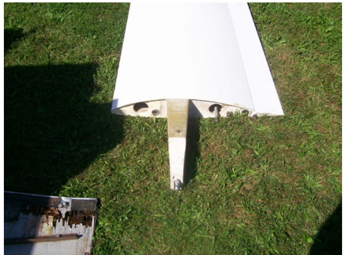
Right wing root showing single spar.
