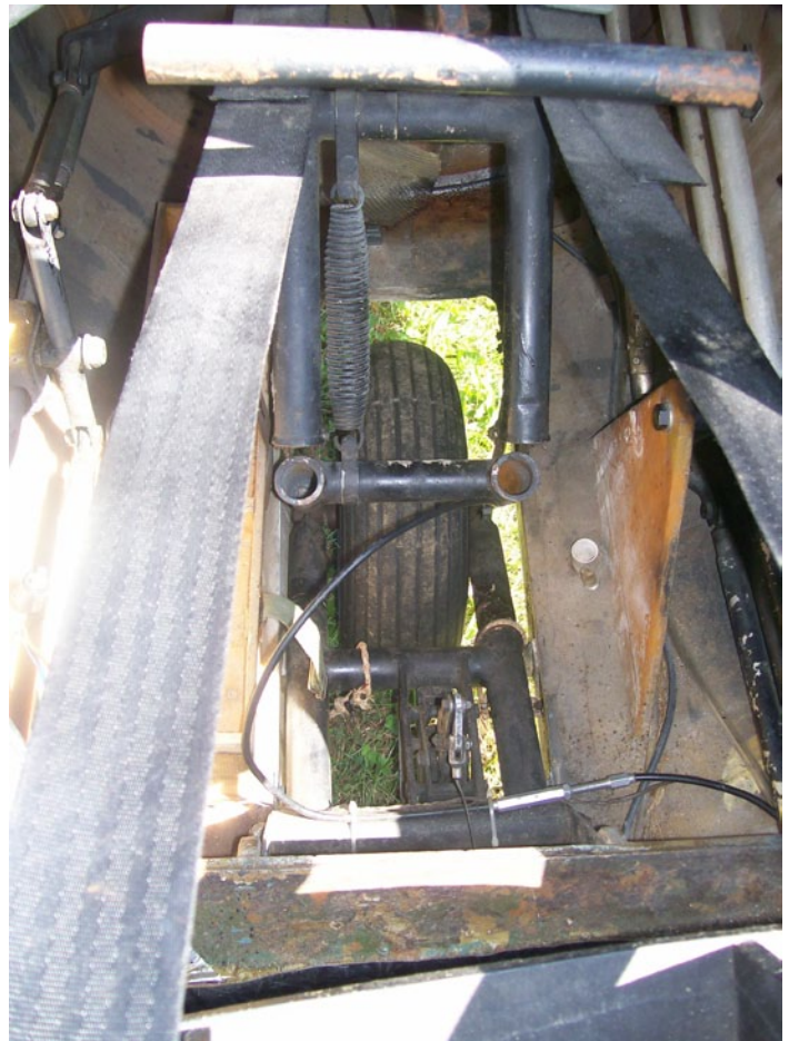
Gear down and locked note tow release and brake cable.
