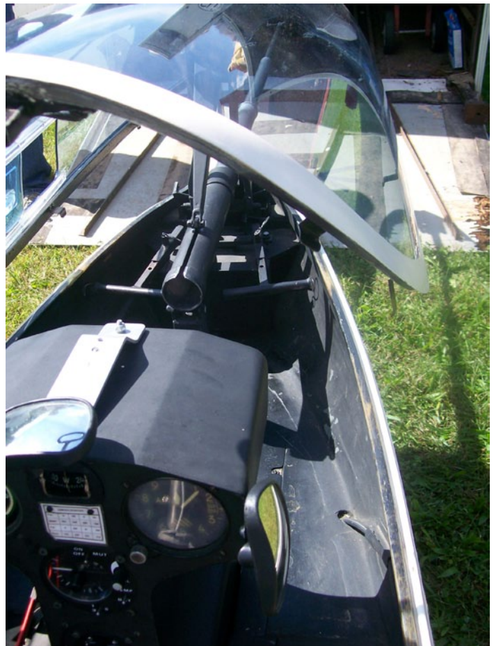
Below: Those T-bars up front are the rudder pedals.
