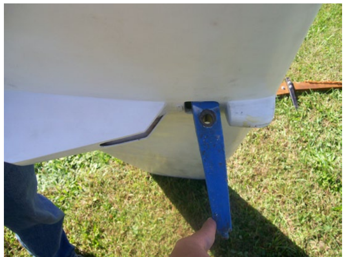
The stab pivots around the hole in the blue lock. Full up.
