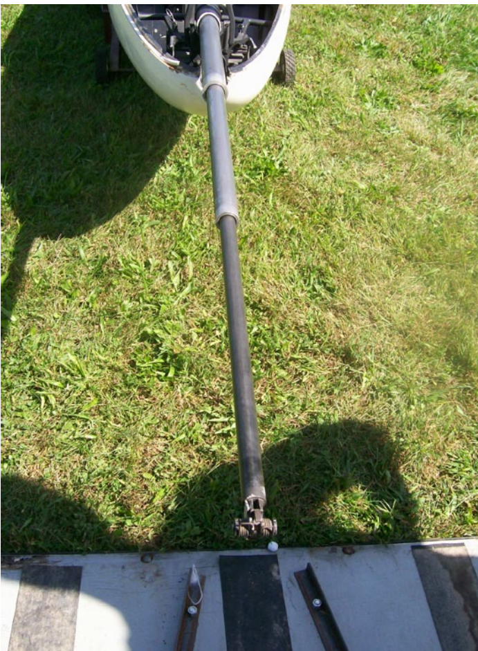
Below: Canopy front retraction and support tube.
