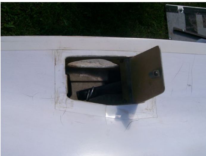
Aileron connection and drive arm.
