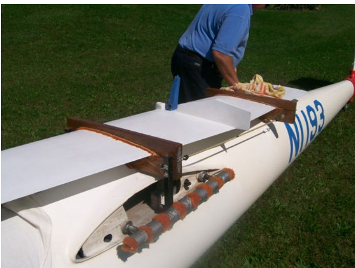
Above: Tow release resting on your left leg flaps extended for tow and spoilers closed and locked.
