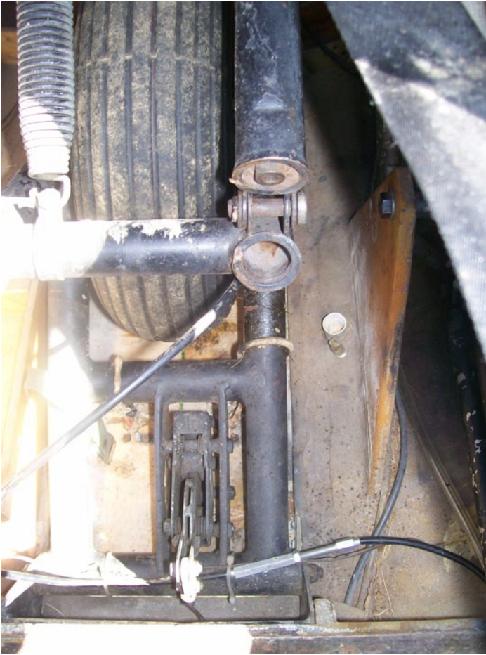
Gear up and locked note off center tow release.
