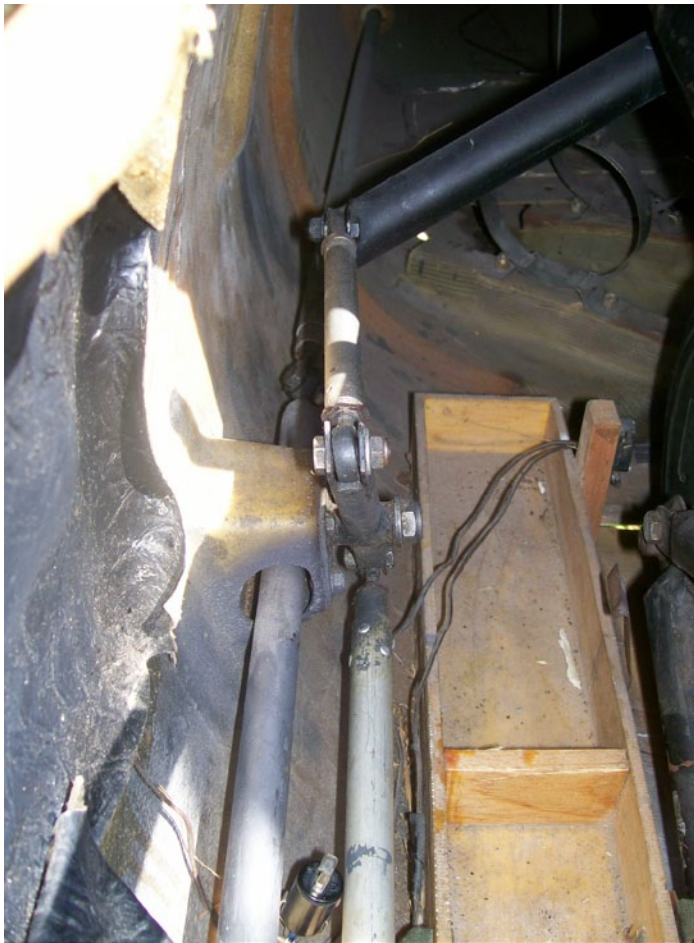
Down in the belly battery box and landing gear retraction arm.
