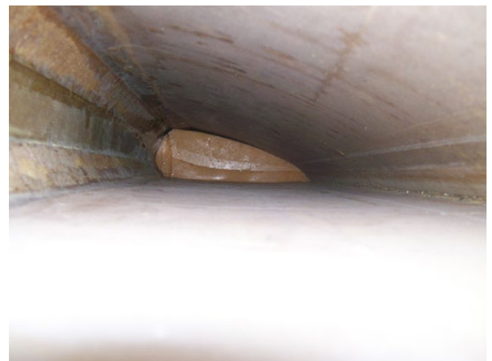
Above: Inside the leading edge of the left wing. Look Ma, no ribs! Wing spar is to the left.
