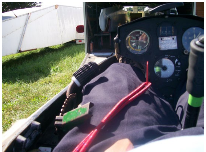
Above: Tow release resting on your left leg flaps extended for tow and spoilers closed and locked.
