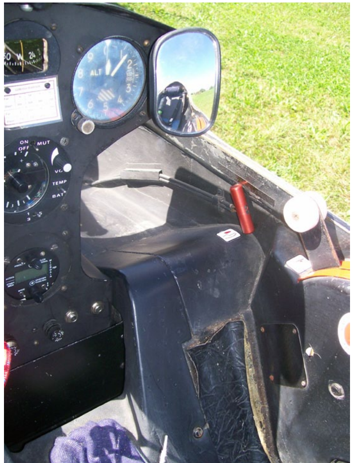
Below: Right side wall landing gear retraction control.
