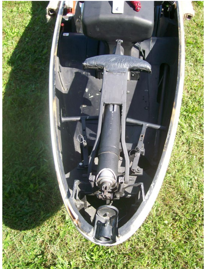
Below: Canopy front retraction and support tube.
