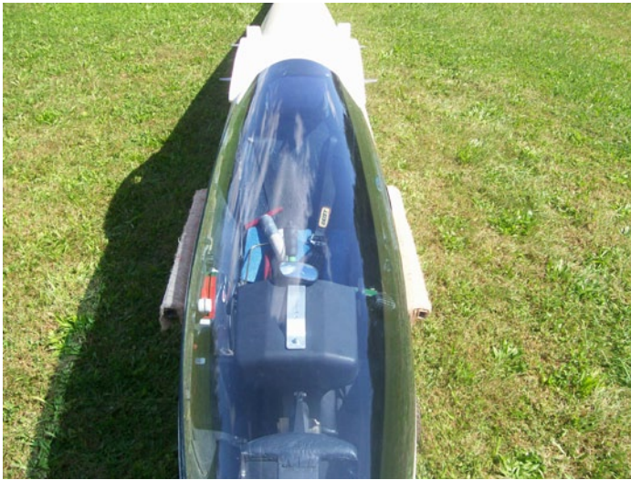
Above: Canopy cover removed while in fuselage dolly.
