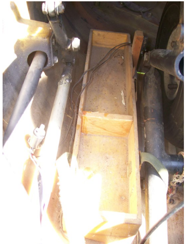
Battery box landing gear retraction and elevator drive rods.
