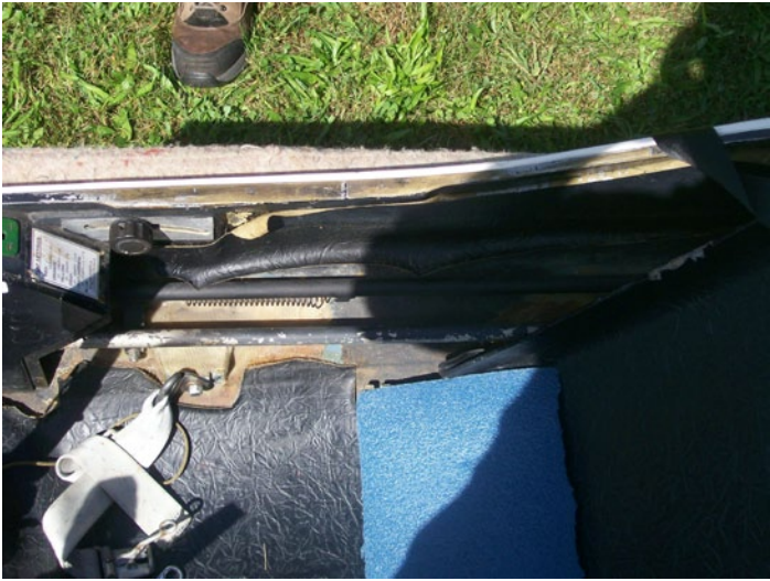
Right arm rest removed exposing landing gear retraction and stab drive rods note trim springs over stab drive.
