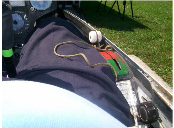
Above: The green cable is canopy jettison followed by the landing gear retraction lever and then by the trim.
