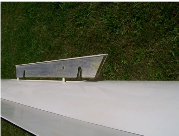
Above, top: Top Right wing showing spoiler extended.
