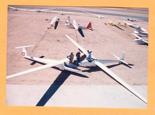
Dan Pearson made a modification to his Diamant 18 by taking off the canopy and installing a fairing over the cockpit tub. Other modifications required to fly "Topless" include the addition of a bulkhead behind the cockpit to prevent the airstream from entering the fuse.
